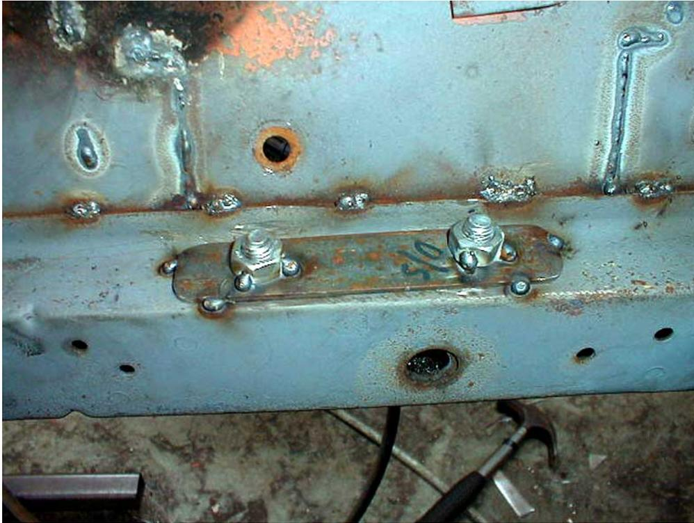
This is potentially good, but tubing not thick enough, and need to grind most of weld away.
