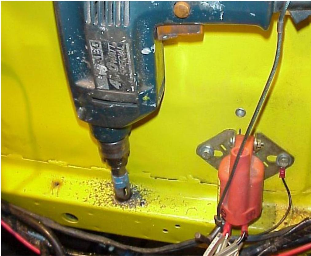
Then I welded washers to cut to length tube spacers [approx 51.5 mm long each]. Incidentally there's plenty of ways to do this but I've sat tubes on top of nuts in chassis rails. I drilled nuts out to suit new bolts.
