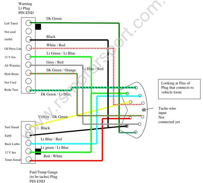
Change the wires in the loom around to the diagram below by carefully removing the pins. They will bend out of shape and need to be bent back a bit before re-inserting them in there new home. The 11 pin plug to the main loom has a red insert that locks all of the pins into it – this insert need to be clipped out first before adding the pins into it. I stole a wire from another loom to connect up the tacho pin.
