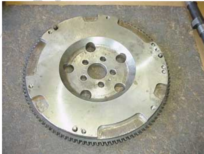
The photo above shows a flywheel made to suit both the 5 bolt Datsun crank, and the Ford Lotus Twin Cam 8.5" clutch. In order to reduce weight five 20mm holes were drilled near the centre, and segments were milled at the periphery of the flywheel. Total weight is around 5.75Kg. EN8 medium tensile steel was used.
