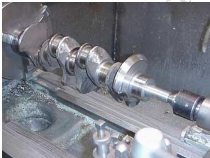
The photo above shows the modifying of a Datsun crankshaft - in this case a L16. The rear of the crank is machined as per the Ford crankshaft.
