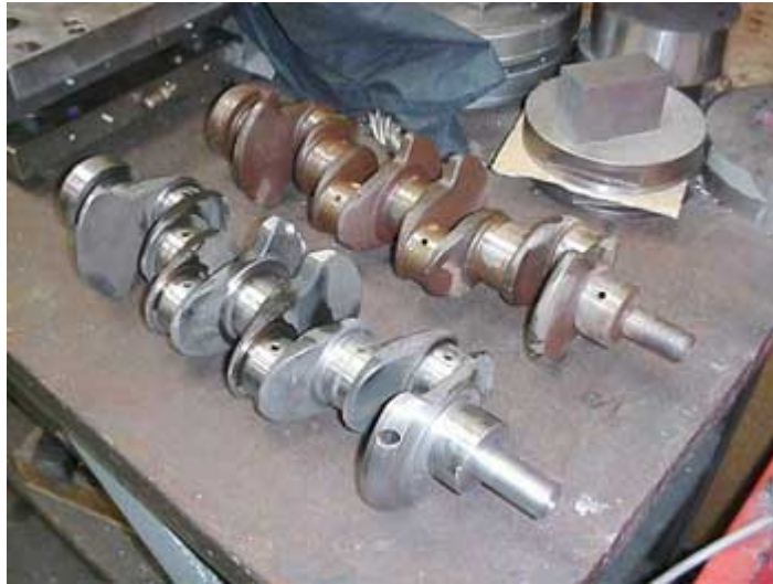
The photo above shows the modifying of a Datsun crankshaft - in this case a L16.
