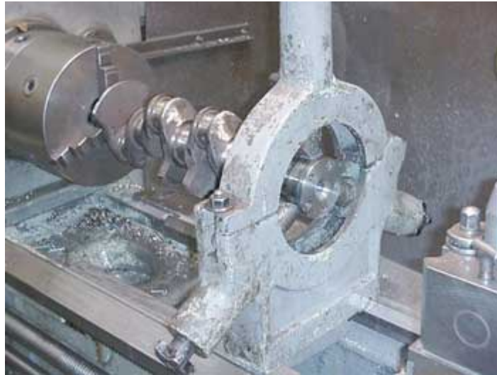
The photo above shows the modifying of a Datsun crankshaft - in this case a L16. The rear of the crank is machined as per the Ford crankshaft.
