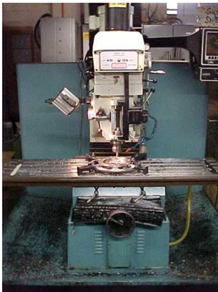
The photo below shows the CNC milling of the six radial slots
