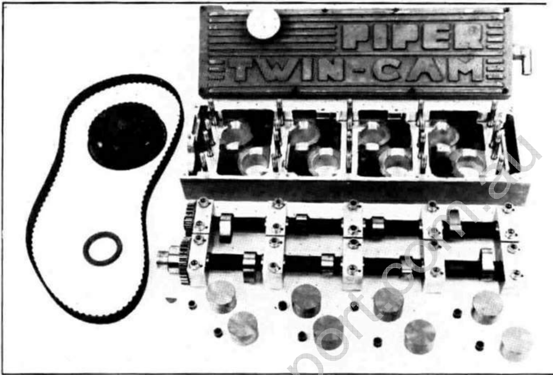
Piper's twin-cam conversion provides even more potential for the Pinto engine.
